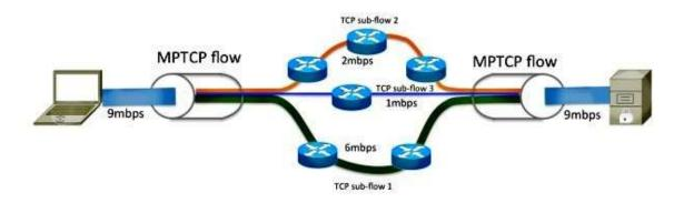
Figure 6: TCP Multipath flow within the FastApn Kernal
