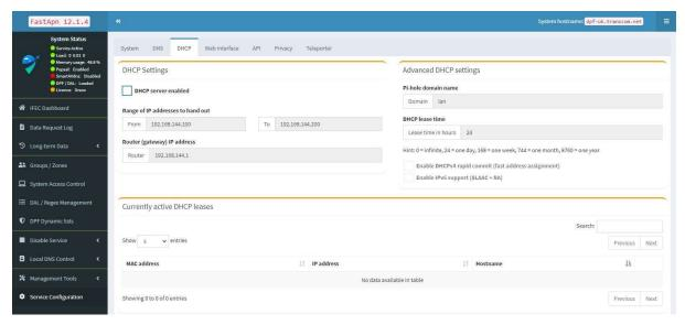
Figure 30: DHCP Configuration including active leases
