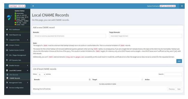
Figure 21: Adding CNAME records to the system
