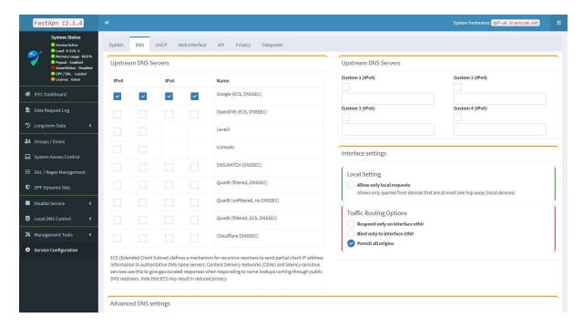
Figure 28: DNS Upstream Configuration - (Unbound Fully Recursive available)
