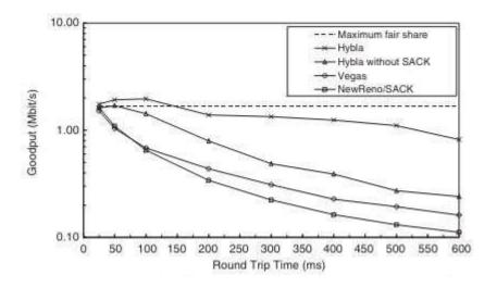
Figure 5: Performance of different TCP versions in the presence of congestion
