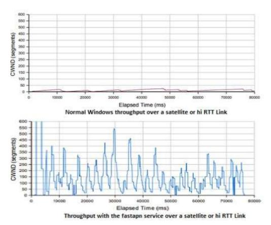
Figure 4: Difference before and after using the FastApn service on a high RTT link
